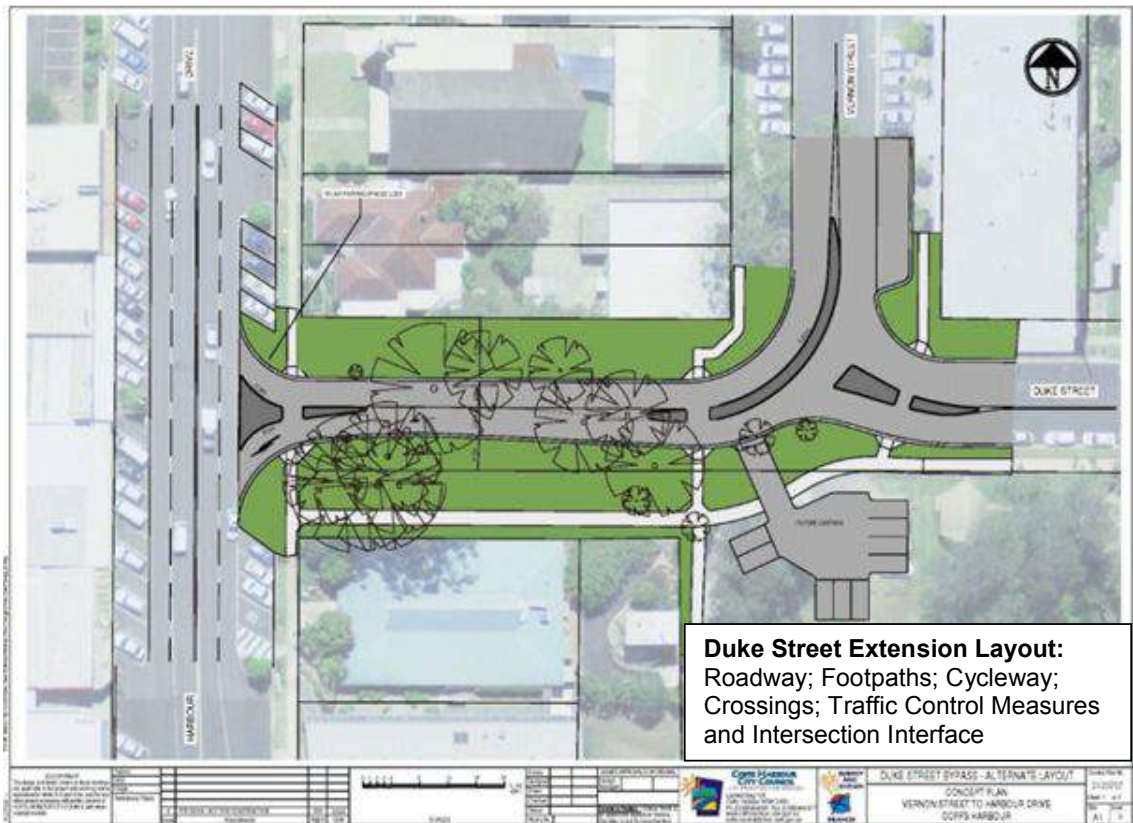
Diagram 4 – Positioning of Pedestrian Access, Cycleway/Footpath, and Crossings. Note Left Out / Left In restrictions at Harbour Drive Intersection.
