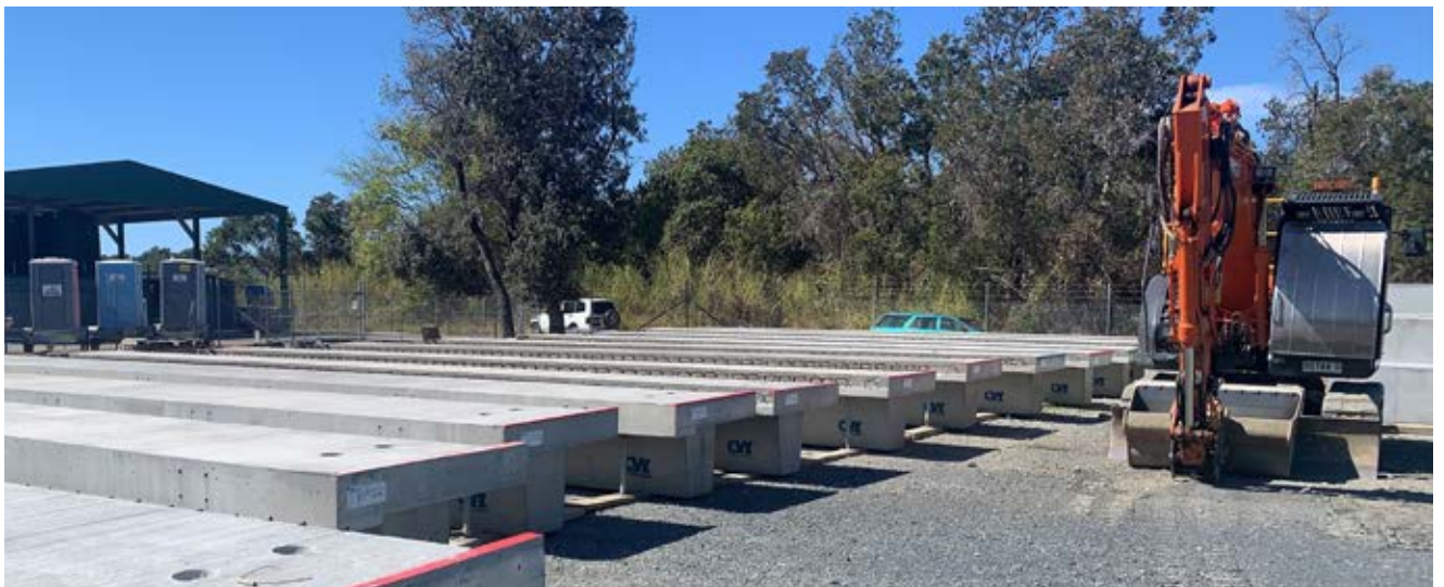
Coastal Works Precast Beams ready for delivery
