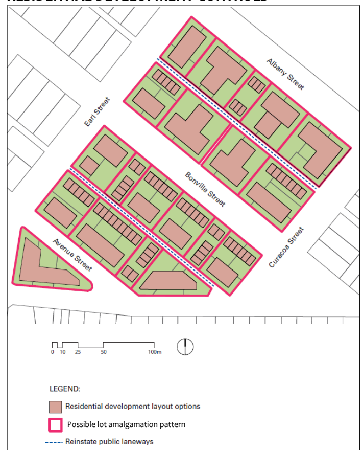
FIGURE 20 - ALBANY STREET HIGH DENSITY RESIDENTIAL DEVELOPMENT CONTROLS
