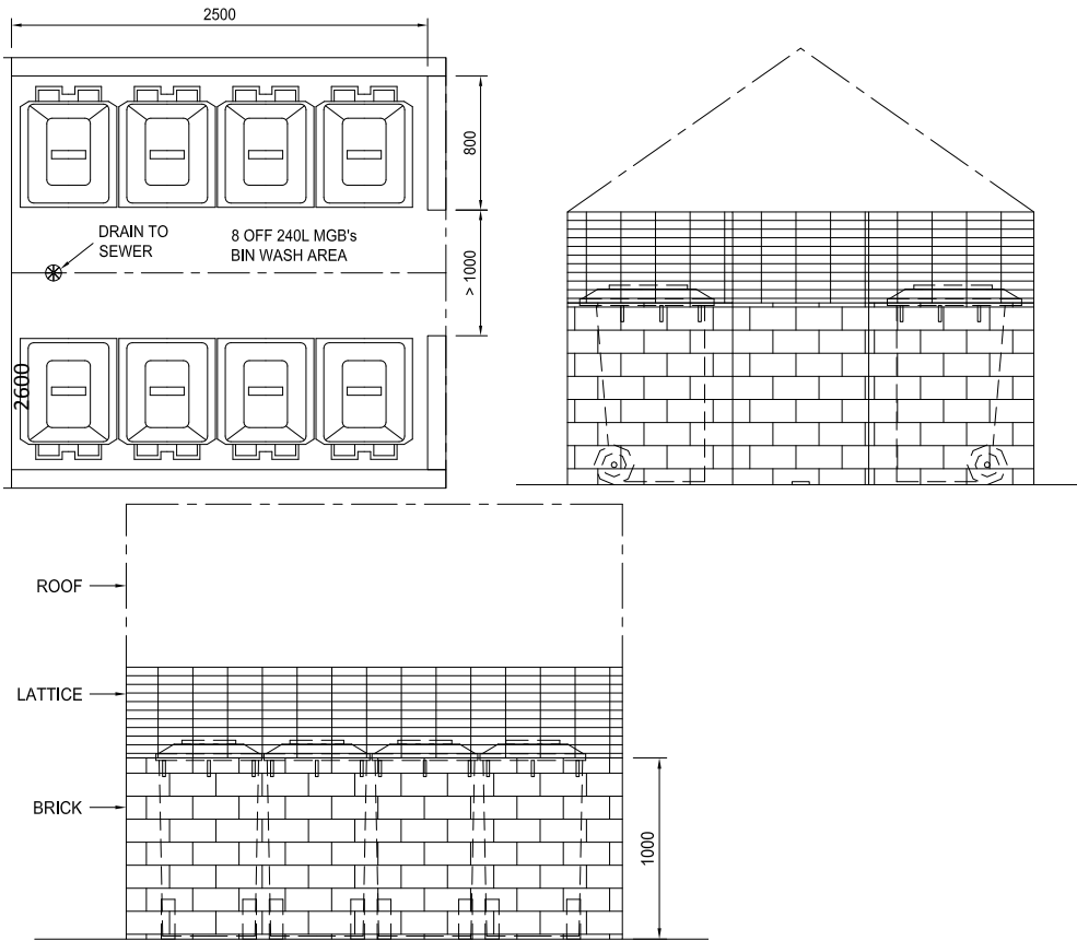
FIGURE A – EXAMPLE ONLY MGB STORAGE AREA (8 MGBS)
