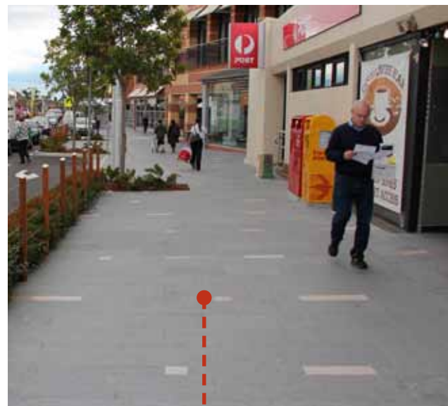
Extend sense of space with simple kerb to building paving pattern with no formal banding
