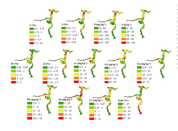
Figure 5. Contents of major elements and trace metals from surface sediment samples around Hearnes Lake. Dots are locations of surface sediment grabs. Red indicates highest contents found, while green areas indicate less concentrated areas. Only Sites 12 and 13 exceeded the ANZECC sediment quality guidelines (SQG) recommended value of 20 mg kg<sup>-1</sup> for As (37.24 and 22.61 mg kg<sup>-1</sup>, respectively, areas in red).
