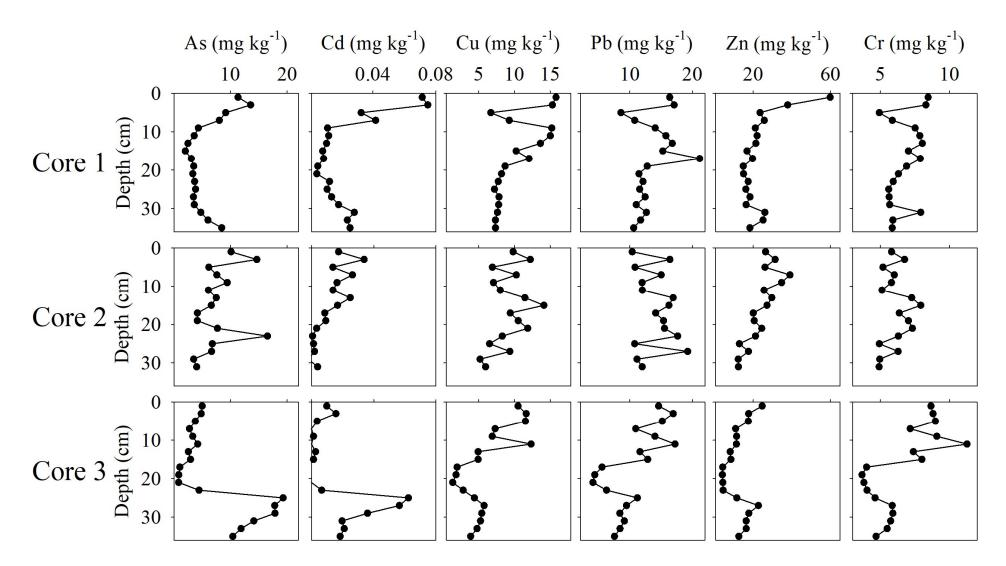
Figure 4. Contents of trace metals plotted against depth from Hearnes Lake sediment cores.
