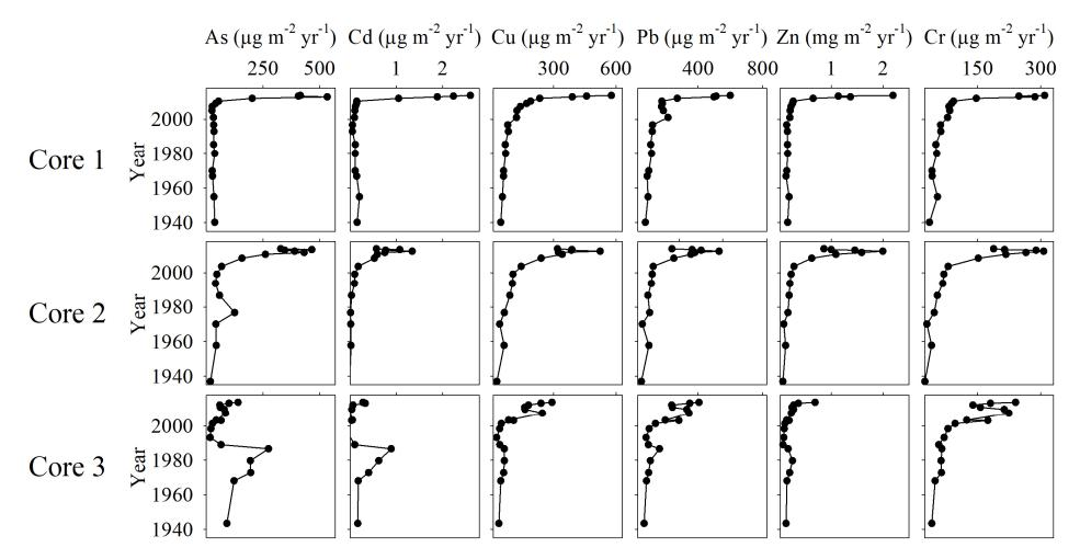
**Figure 7.** Sediment flux of all elements compared with sediment ages from Hearnes Lake sediment cores. Flux calculated as amount of contaminant present in sediment times sediment mass accumulation rate calculated using <sup>210</sup>Pb radionuclide counting. Flux values represent amount of contaminant entering sediment per area per time (µg m<sup>-2</sup> yr<sup>-1</sup> or mg m<sup>-2</sup> yr<sup>-1</sup> as denoted).
