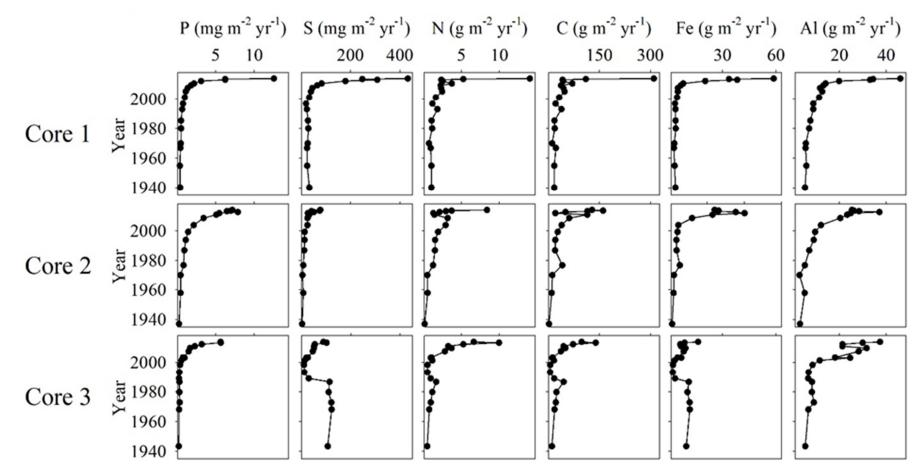
**Figure 7 (cont.).** Sediment flux of all elements compared with sediment ages from Hearnes Lake sediment cores. Flux calculated as amount of contaminant present in sediment times sediment mass accumulation rate calculated using <sup>210</sup>Pb radionuclide counting. Flux values represent amount of contaminant entering sediment per area per time (mg m<sup>-2</sup> yr<sup>-1</sup> or g m<sup>-2</sup> yr<sup>-1</sup> as denoted).
