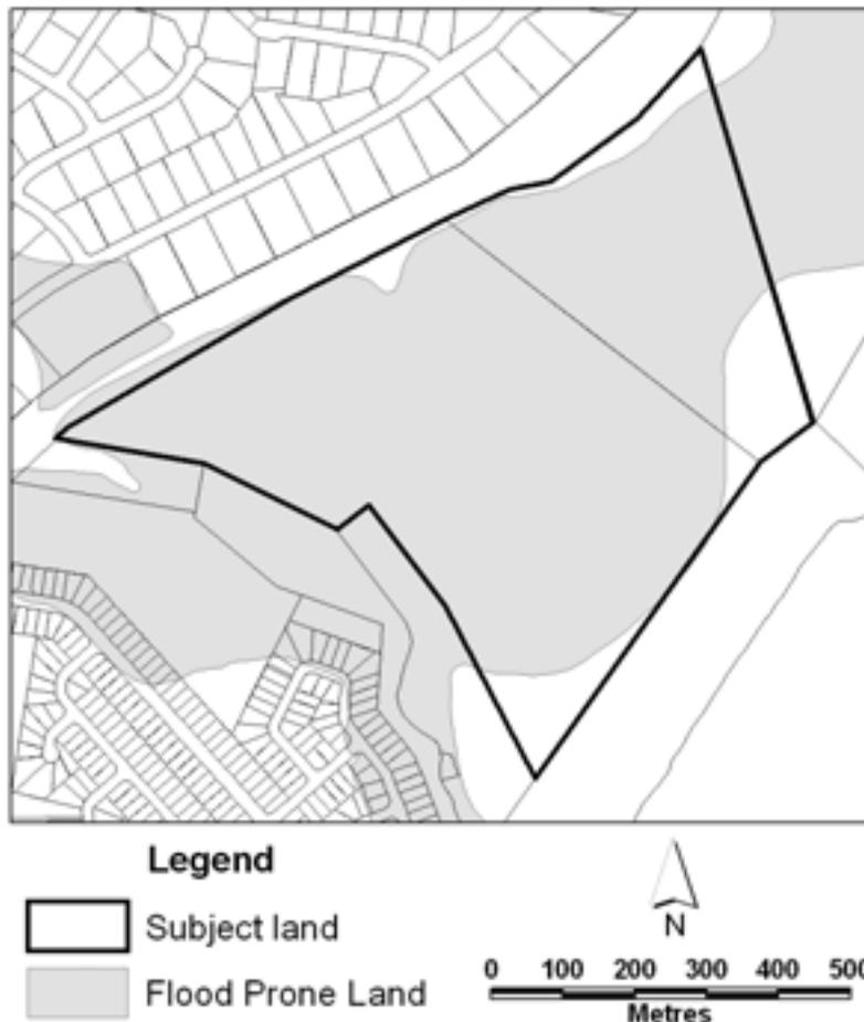
It is clear from this map that residential development of the land would be severely limited given the extent of impacts caused by flood prone land. Filling to avoid flooding would create new problems in relation to water movement and may create adverse impacts on adjoining land.
